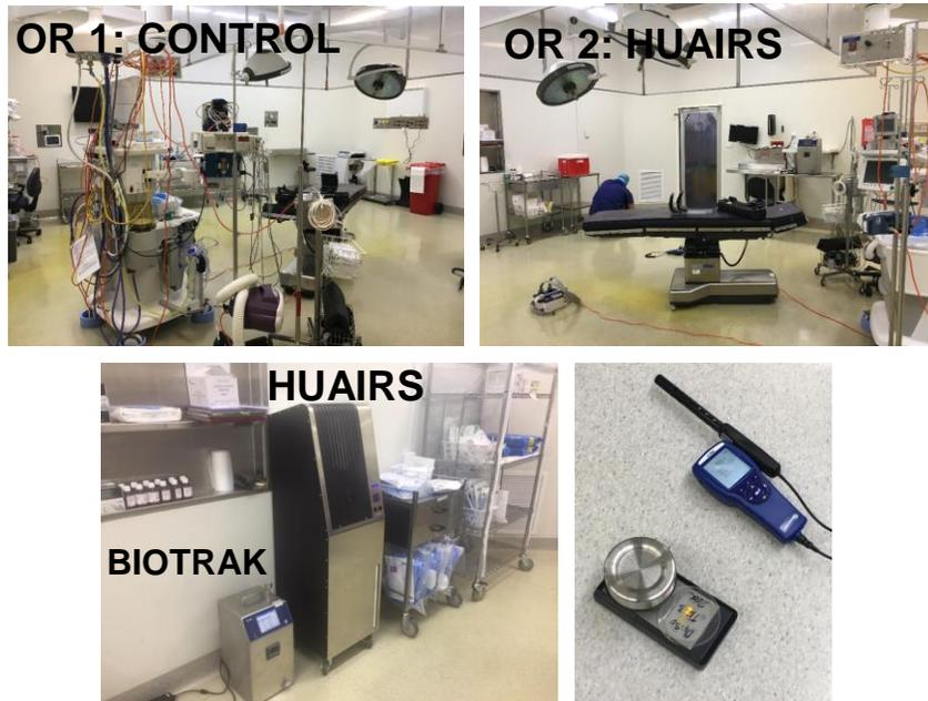
ORs evaluated in the study (Top). Viable and non-viable particles were measured using the LIF (BIOTRAK) with and without the HUAIRS system. Standard air sampling and agar plates were used for bacterial counts.
