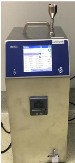
LIF (BIOTRAK) was used in this study to monitor viable and non-viable particulate.
