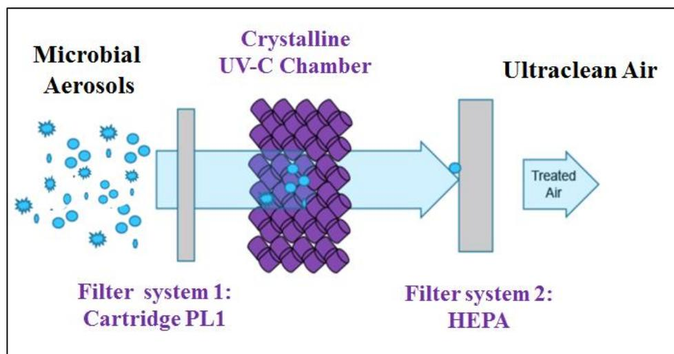
**Figure 1.** Mechanism of ultraviolet activation in HUAIRS system
