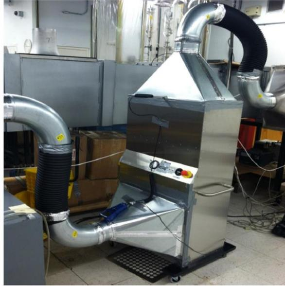
**Figure 2.** View of the ESP unit installed in the test duct. Air flow in the test duct is from left to right.
